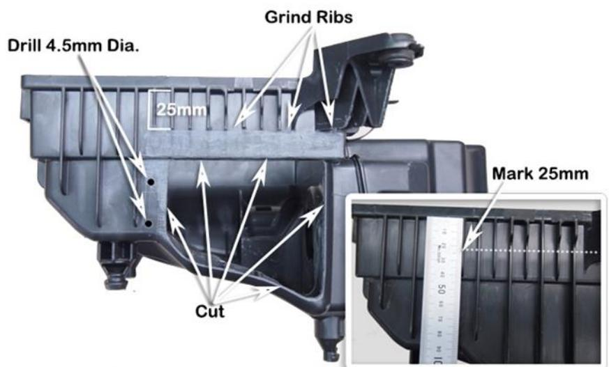
Using a body saw or die grinder remove the ribs as shown.
