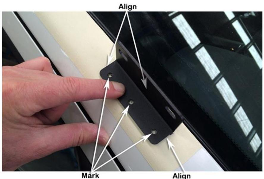
Drill a pilot hole at each of the three marked hole positions. Drill each hole position to 8mm diameter with a step drill or 8mm drill bit.
