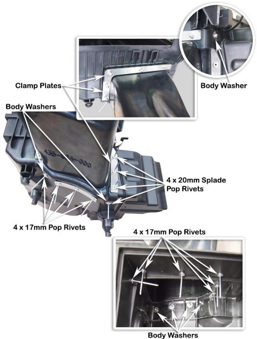
With all pop rivets, clamp plates and body washers in place, secure all pop rivets using a pop rivet gun. Clean-up any excess sealant to ensure a neat finish.
