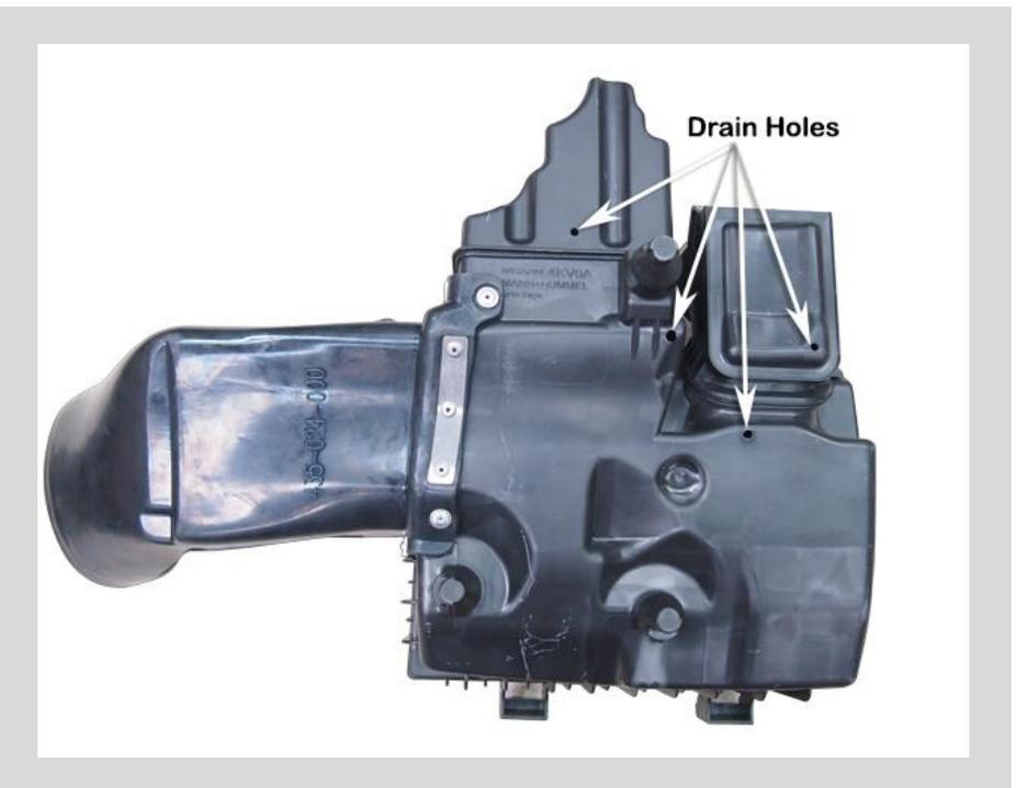
32 Install the air cleaner base and hose assembly into the vehicle. *Hint: squash the end of the hose whilst installing through the hole in the inner guard.*
