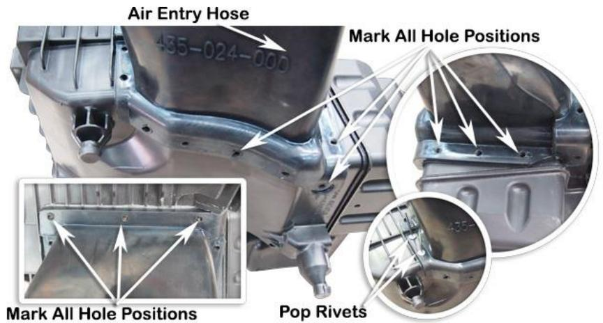
Remove the hose and drill the twelve marked hole positions with a 4.5mm drill bit.
