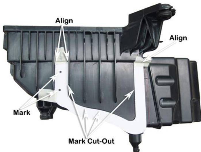
Using a body saw, remove the marked cut-out section of the air cleaner base.
