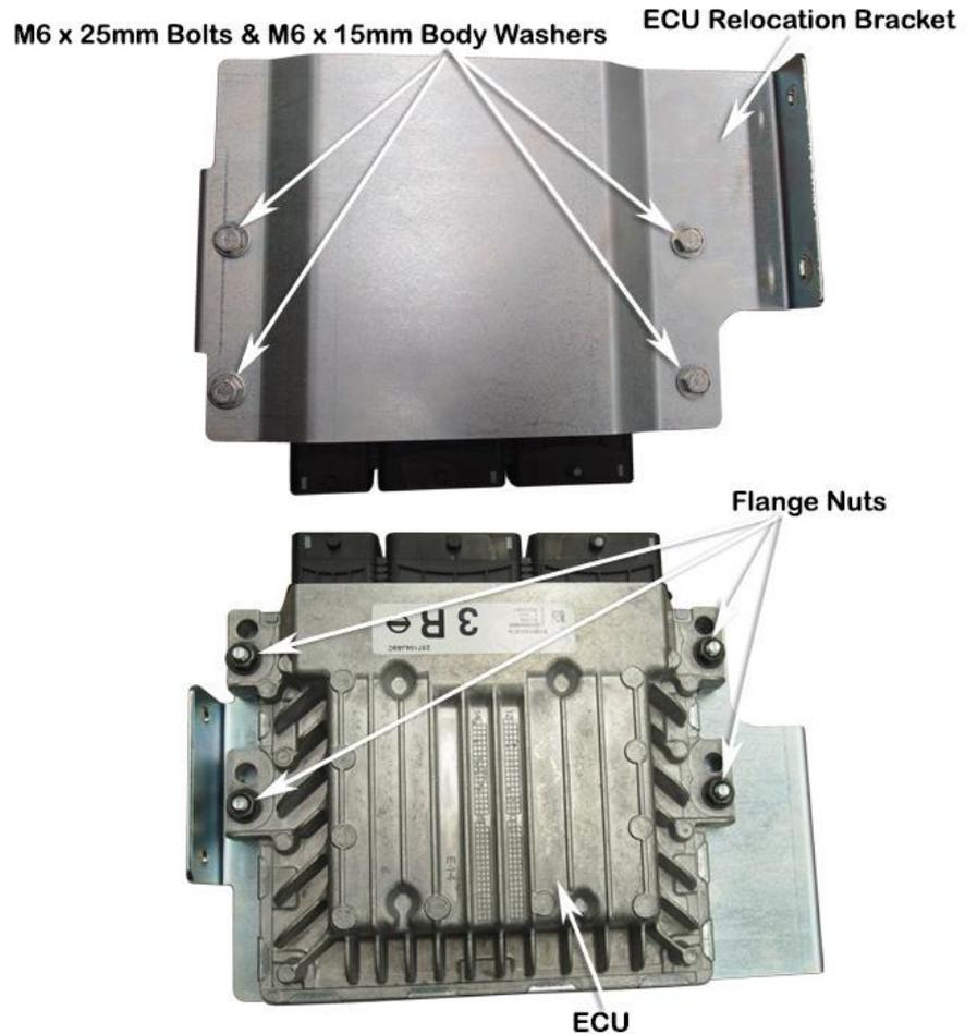
Assemble the idle control module to the relocation bracket (item 24) with three 6.0mm x 20mm hex bolts, (item 27) and three 6.0mm body washers (item 29), install the bolts with washers installed through the bracket, install two 6.0mm body washers to each of the bolts for spacers, and install the idle control module. Install a 6.0mm body washer and a 6.0mm nyloc nut (item 30) to each of the bolts.
