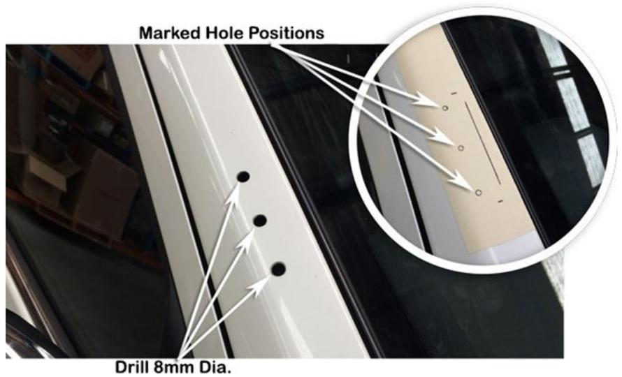
Install the plastic inserts (Item 6) into the 8mm diameter holes in the A-pillar.
