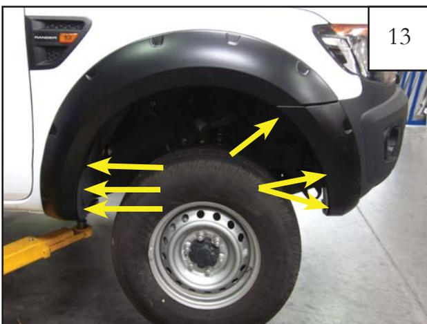
While holding Front Flare/Bumper Piece Combo on Vehicle start six (6) supplied Screws (SW1-0056) into flare and into clips installed in steps 10 & 11.
