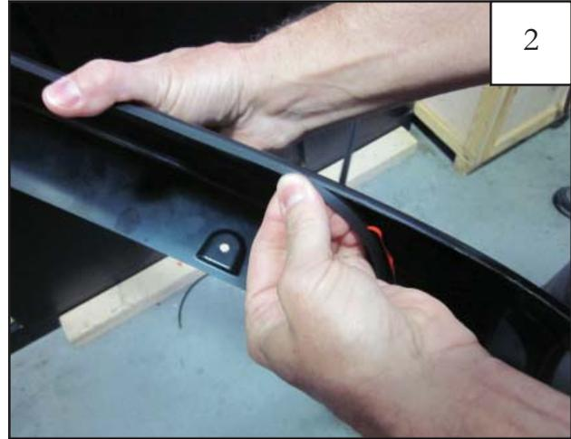
Press edge trim into place along the top edge of the flare in one-foot increments, pulling red vinyl backing free as you continue to work your way around the top edge of the flare.
